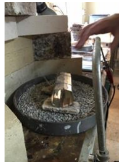
Getting ready to Solder Bob's pitcher. Binding wire holds it in place
