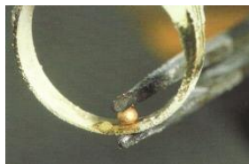
Figure 7.4. Sweat soldering a bead in place
